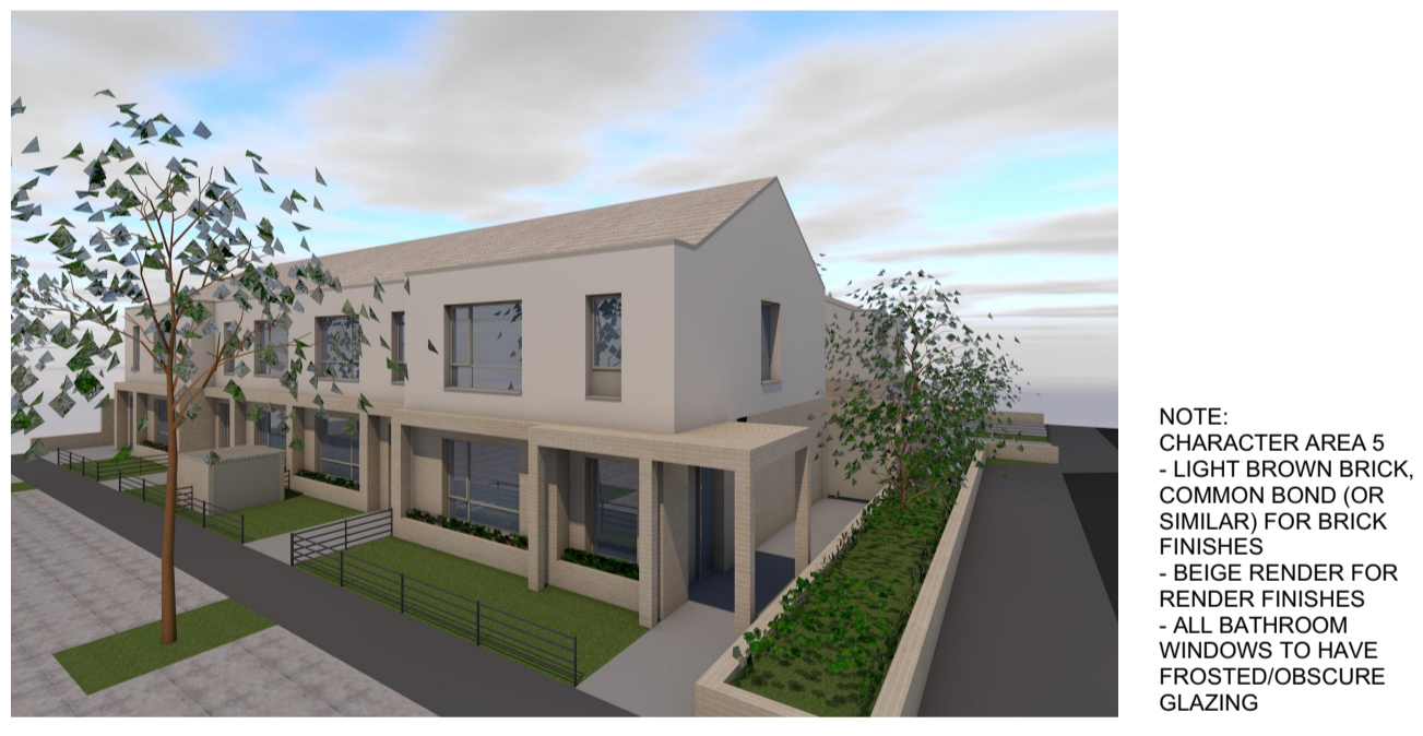
AXONOMETRIC VIEW SHOWING A TYPICAL CORNER CONDITION
